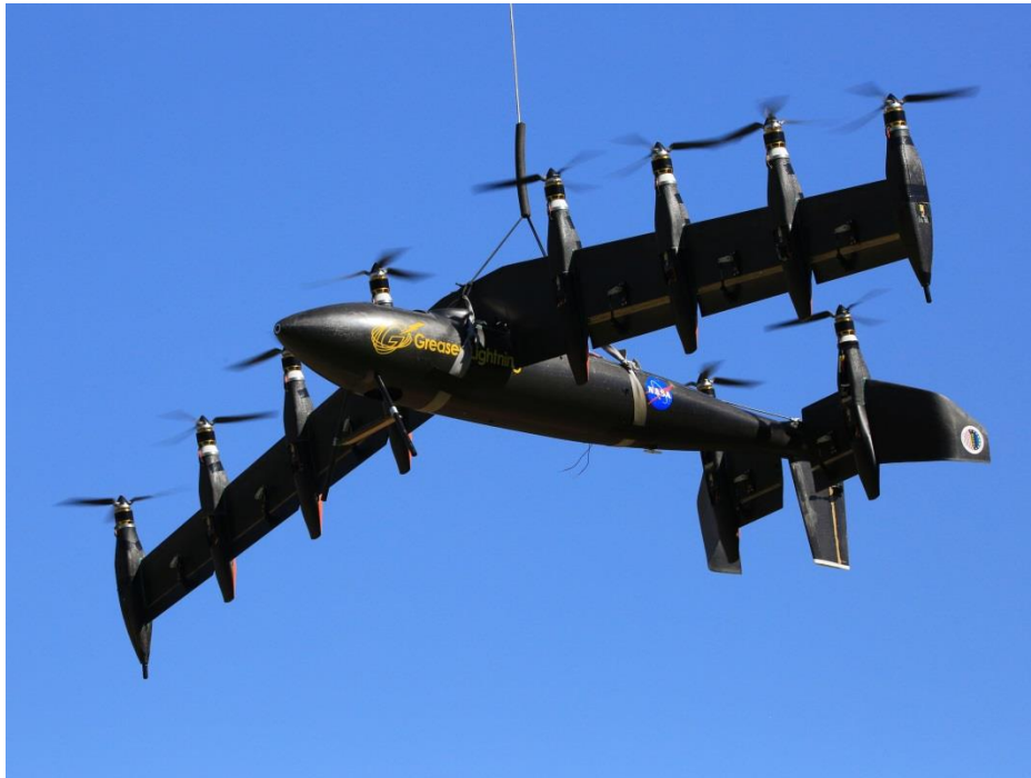
Figure 20-4: NASA Electrically Powered UAV Conducting Hover Tests.
